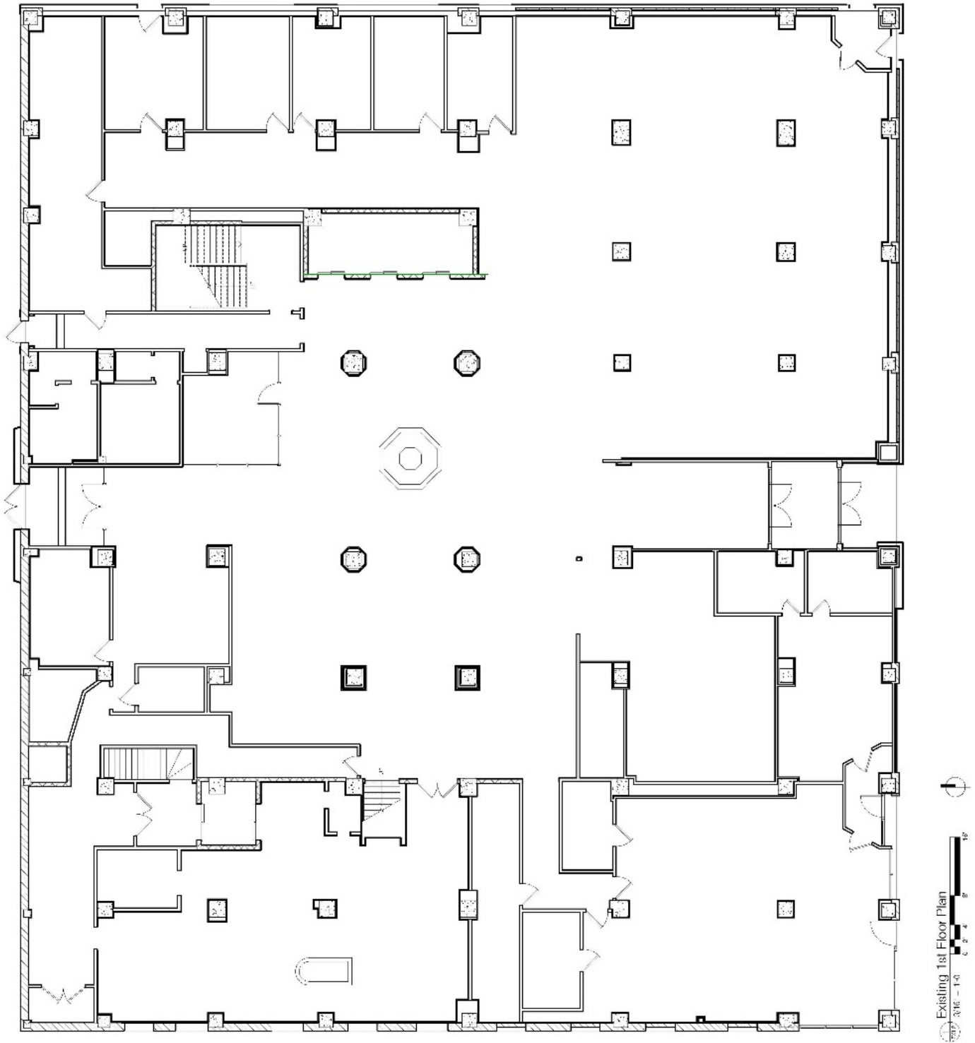
Figure 19. Existing Second Floor/Mezzanine Plan
