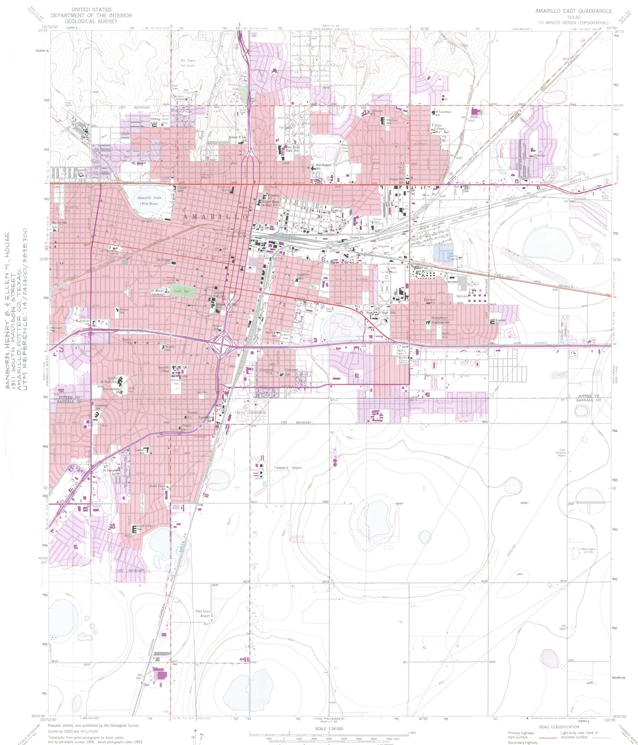
Polyconic projection. 1927 North American datum 10,000-foot grid based on Texas coordinate system, north zone 1000-metre Universal Transverse Mercator grid ticks, zone14, shown in blue
